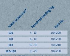
\* Data refers to HEUER Vices. Also suitable for other makes provided that permitted loading weights are observed. When ordering please do not forget details of make and size.
